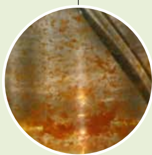
iron ions form insoluble precipitations in the alkaline liquor
