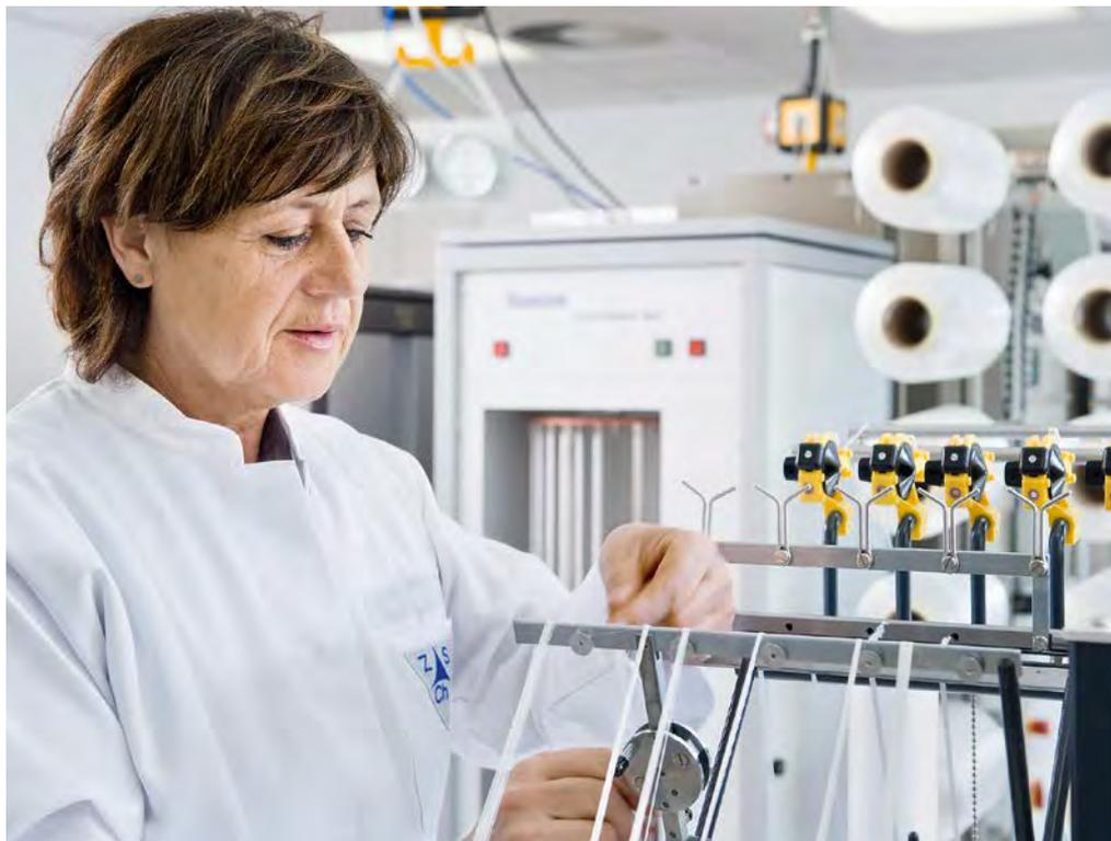
▷ Our measuring technology enables us to determine various textile parameters that are important for the performance of our products. Here: preparing a yarn count measurement.
