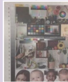
Coated using 10 Meyer Rod on PET film, dried at 70 °C, then placed over internal clarity standard
